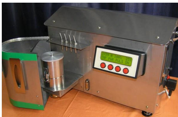
Fig.5. Dynamic processing microwave reactor, concept at the INCDTIM-Cluj Napoca
