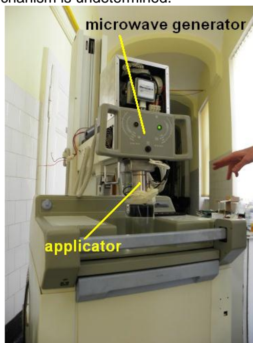
Fig.3. Hyperthermia installation with six axis freedom frame, using the CW microwave generator
